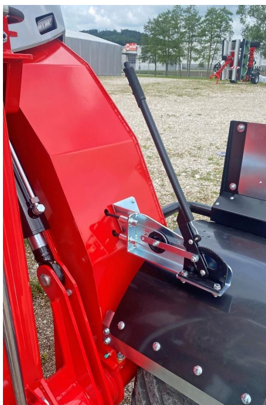
Mechanical parking brake (left machine side)
