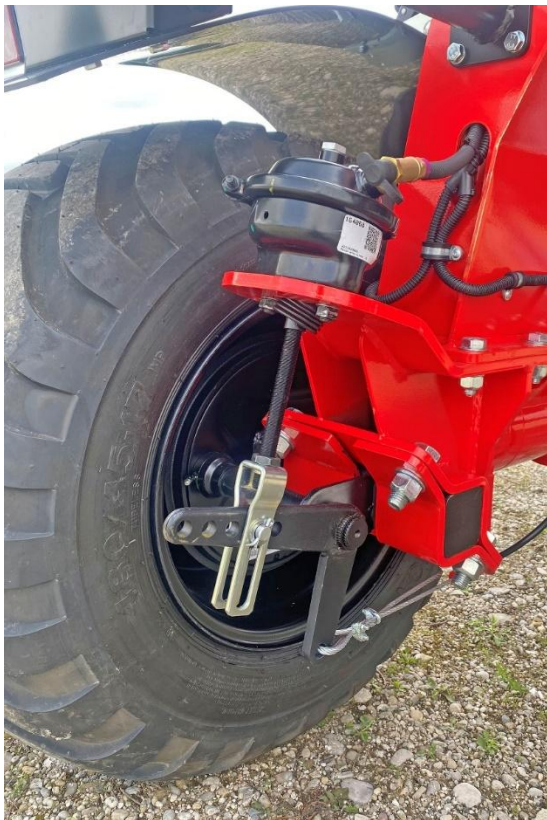
Brake axle with air brakes
