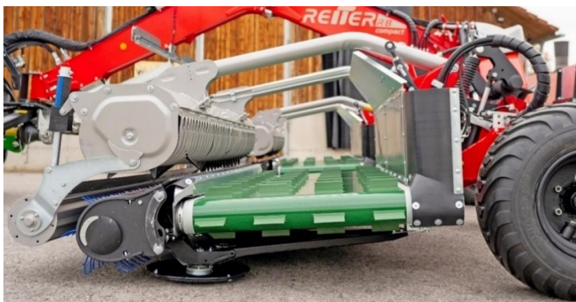
Highest position approx. 3.0 cm raking height
