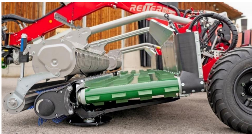
Lowest position approx. 0.5 cm raking height
