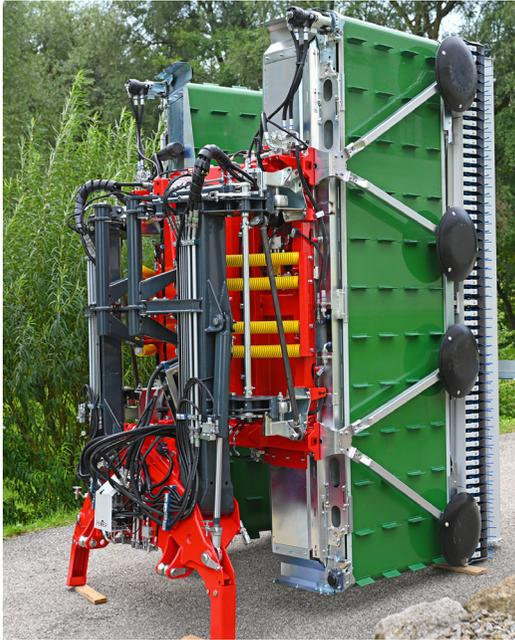
The robust folding frame is mounted very short, so the centre of gravity is close to the tractor. The hitching is carried out via double-cut lugs cat. A centring aid facilitates coupling.
