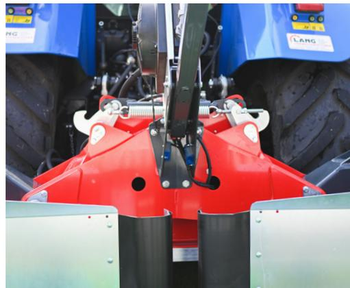
Mechanical transport lock of the outriggers
